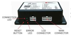
The WiFI module now comes with a WiFi to REC 2Q cable but if you need to reuse your existing cable, you can cut off the the DB9 connector and crimp on pins and use a 6 pin connector as shown here
