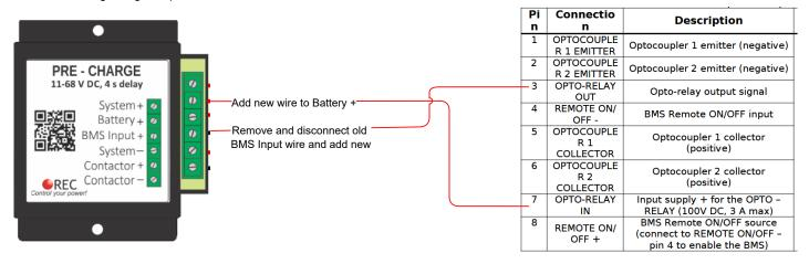
See REC 2Q Quickstart manual for connecting your other optocoupler outputs
